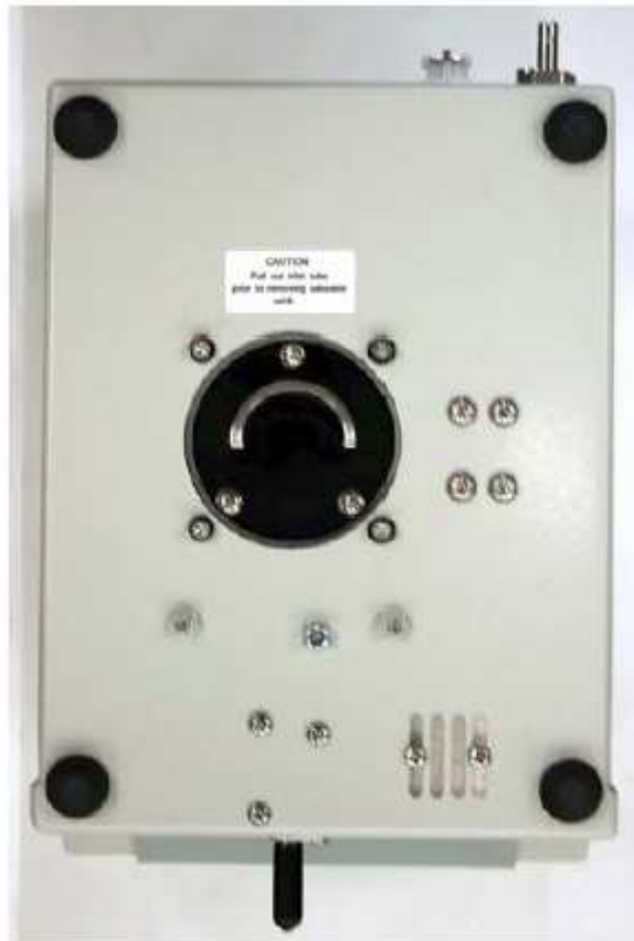
Figure 3-4 Bottom Panel Showing Removable Saturator Base
